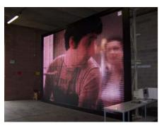
Large out door mega screens are made up of many thousand LED's arranged in RGB formation. Once assembled these banks of LED's need to be potted for two reasons
